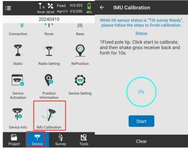
You could follow the operation steps of IMU Calibration and then the IMU will be calibrated.
